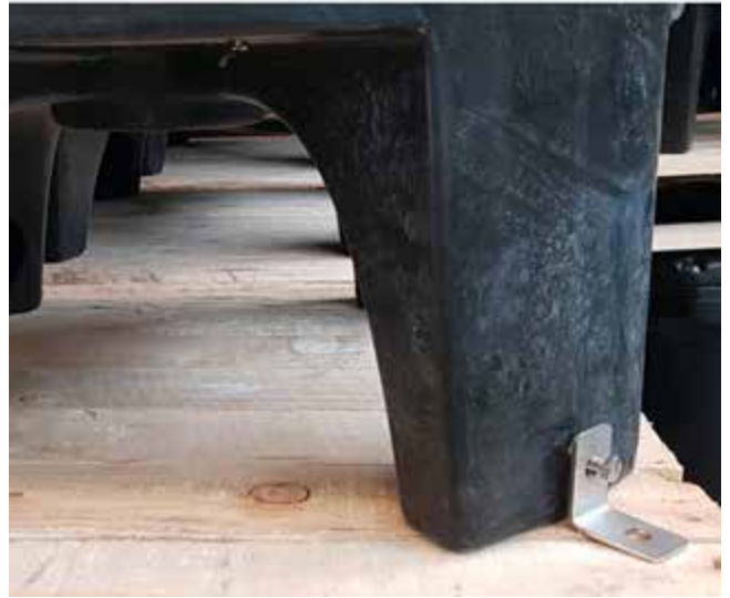
Figure 4 - Bolting the feet
